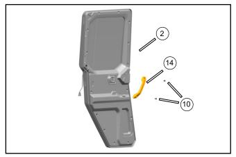
Use the inner hexagon bolt M6×20 (10) to mount the LH & RH inside armrest (14) on the LH & RH rear door assy (2).
