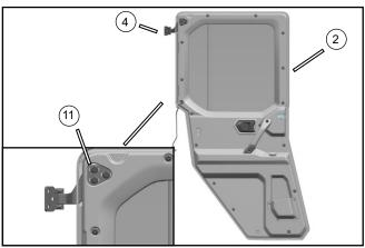
Finger-tighten the hexagon flange bolt M8×16 (11) to secure the LH/RH rear upper hinge assy (4) on the LH/RH rear door assy (2).
