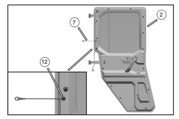
// Use the steped bolt M6×17 (12) to mount the limiting cable assy (7) on the LH/RH rear door assy (2).
