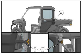
Place the LH/RH side door assy in the frame area, pass the lower hinge through the plate (a) hole, secure the bolt of the upper hinge (4) and lower hinge (3), at last mount the plate (a) on the vehicle body.
