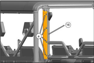
Place the LH/RH seal baffle (16) in the assembly area, use the hex steped bolt M6×14 (a) to finger-tighten it.
