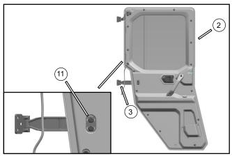
Finger-tighten the hexagon flange bolt M8×16 (11) to secure the LH/RH lower triple clamp assy (3) on the LH/RH rear door assy (2).
