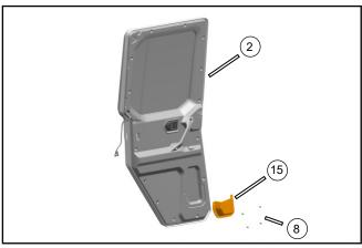
Use the self-tapping screw ST4.8×16 (8) to mount the LH & RH rear door glove box cover (15) on the LH & RH rear door assy (2).
