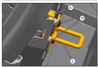
Place the rear door fastener assy (5) and buckle bracket assy (6) in the assembly area, use the inner hex screw (10) to mount them on the vehicle body.
