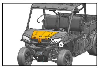
// Disassemble the front top cover (A).
