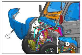
Loosen the rubber buckles (A) on the LH and RH side, open and rotate the front top cover (B) to the position as shown.
