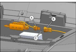
Insert the extension power main body terminal (A) to the terminal of main cable (B), then fix them at location (C). The installation is complete, reinstall the front top cover.
