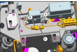
Insert the extension power main body terminal (A) to the terminal of main cable (B), then fix them at location (C). The installation is complete, reinstall the front top cover.
