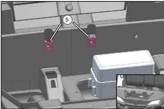
// Install the nut clip M6 (5) at the position as shown.
